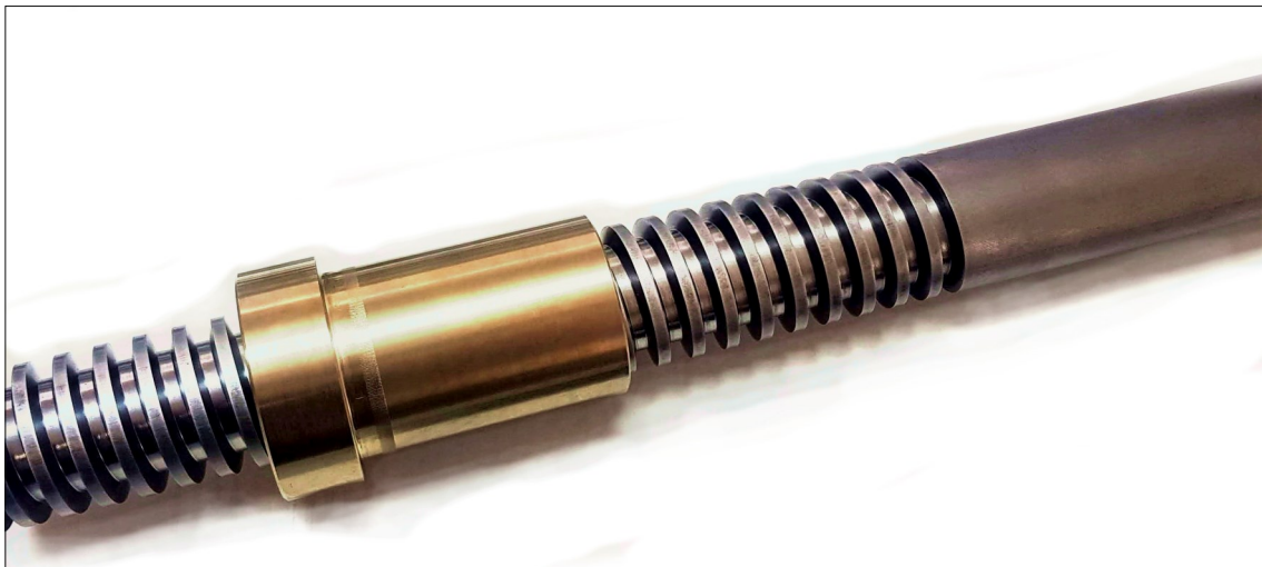
Example of bronze nut with threaded bar TR 50x12 with cylindrical shank of the same nominal diameter of the threaded part
